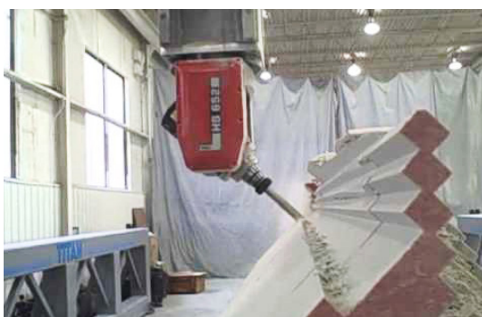
CONTEMPORARY TECHNOLOGY: CNC router machines bespoke red concrete moulds from foam
